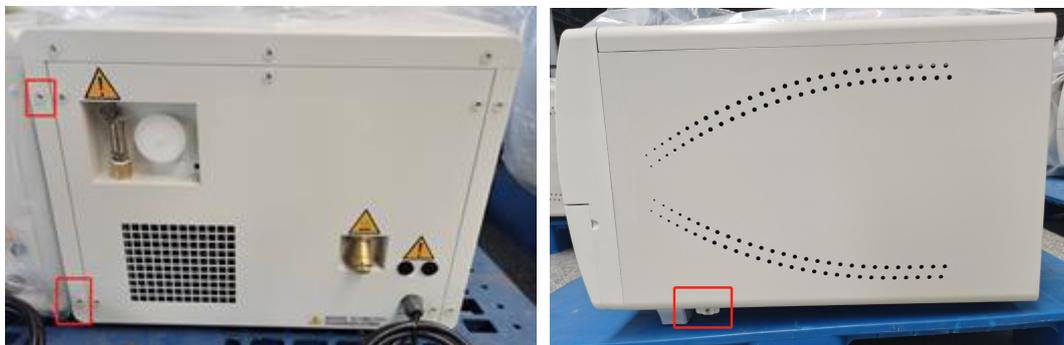
Remove the screws in the red boxes by a screwdriver to uninstall side cover of the device.
