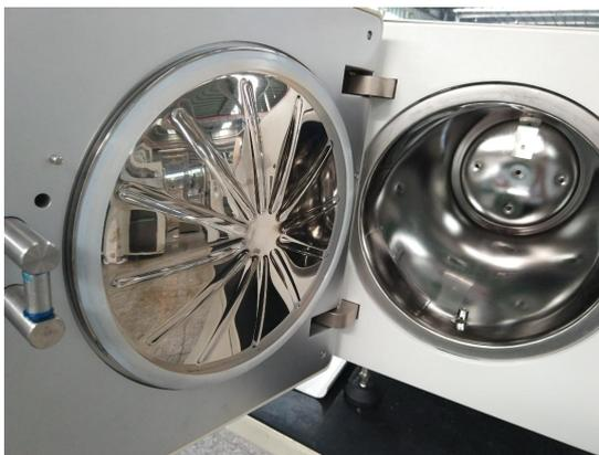
After pulling the door motor hook in step (2), the door is unlocked, and the door can be opened directly in front of the device.
