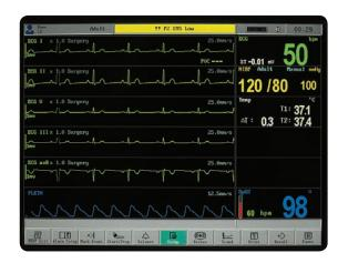
The **Omni (K)** $^{\text{TM}}$  offers a 3, 5, and 12 lead ECG platform. Arrhythmia detection and ST are also standard and measurable on all lead sets.
