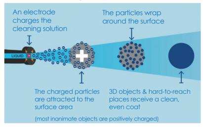
Electrostatic spray technology is one professional fix that uses an electrical charge to allow the appropriate sanitizers and disinfectants to wrap around and evenly coat all types of surfaces for a more complete deeper clean and thorough coverage.
